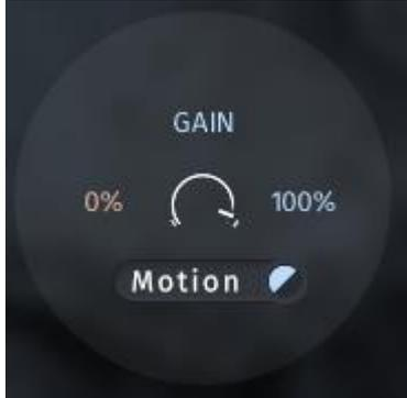
At the heart of our effects lies our MOTION ENGINE that adds movement and depth to the presets. Beneath almost all of the available effects you can find the motion button. When activated the corresponding parameter is controllable with the mod wheel or one of the two other controllers.
