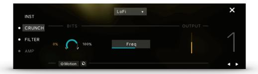
**Bits:** Re-quantizes the signal to an adjustable bit depth. Fractional bit levels (such as 12.4 bits) are possible and can add considerable "grit". Audio CDs have a quantization depth of 16 bits, old samplers frequently used 8 or 12 bits, and 4 bits evoke memories of countless irritating children's toys.
