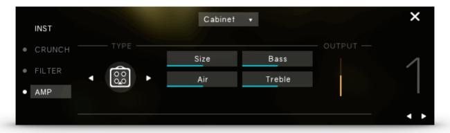
**Type:** Allows you to choose the simulated cabinet model via the left and right buttons or by clicking on the amp symbol.
