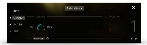
**Shape:** Adjusts the transfer curve. A negative setting results in a characteristic that will expand the signal — lower sample values will be attenuated, higher values will be amplified. Positive settings do the opposite and thusly simulate the compression-like saturation of an analogue circuit. At a value of 0.0, the signal will pass the module unprocessed.
